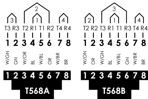
Figure 1: Wiring Schemes
