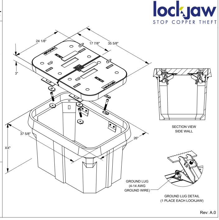
PCA2436 \_ \_-LJ\_ \_ PCX POLYMER CONCRETE ASSEMBLY
