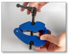
The UTQC-1263 Utility Cable Stripping Stop Clamp allows for quick and precise clamping on medium voltage electrical utility cables ranging from 1/2" to 2-1/2" in diameter. Made from corrosion-resistant anodized aluminum and black-oxide coated steel, it serves as a reliable clamp to stop jacket stripping tools, such as our UTST-1860, from continuing to strip the cable.
