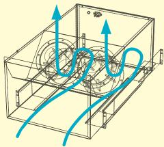
The Lake Effect server enclosure utilizes high performance van axial fans. These highly sophisticated fans were originally designed for the aerospace industry, which
