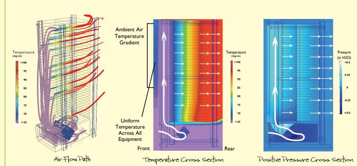
3D Computational Thermal Analysis was independently tested and verified using computer models coupled with powerful fluid dynamic software that predicts airflow and heat transfer in and around electronic equipment. Thirty-six IRMU servers dissipating 10,000 watts total (as shown).
